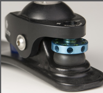
Adjusting Stride Control down will allow for a firmer heel response.
