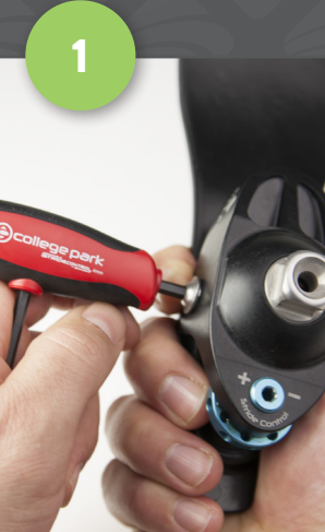
Remove the 4mm axial pin screw...
