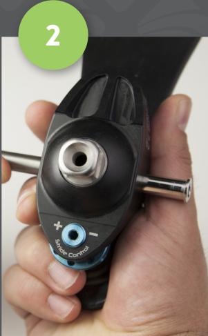
Push the axial pin out with the PinGuide...
